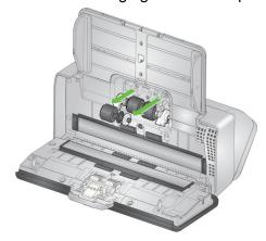
4. Reinstall the urging roller, aligning it correctly.
