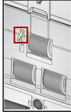
3. Remove the urging roller, then clean it with a roller cleaning pad.
