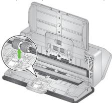
4. Install the new separation roller by aligning the tab with the slot and snapping it into position.
