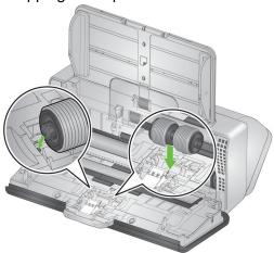
7. Reinstall the pre-separation pad by aligning the slots with the holes on the pre-separation pad and snapping it into place.
