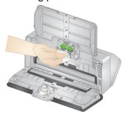
6. Inspect the feed rollers. If the feed roller tires show signs of wear or damage, replace the feed roller. See "Replacement procedures" on page 28 for more information.
