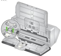
3. Grasp the separation roller and pull it straight out.
