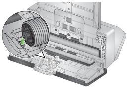
5. Re-install the pre-separation pad by aligning the slots with the holes on the pre-separation pad and snapping it into place.
