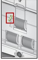
NOTE: Be careful not to damage the paper present sensor when removing or cleaning around the feed roller.
