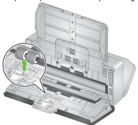
4. Wipe the separation roller tires with a roller cleaning pad. If there are grooves in the tires, wipe in the direction of the grooves. The tires on your model may look different than the tires in this illustration.
