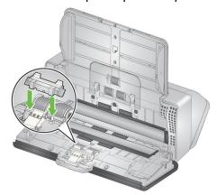
4. Go to *Maintenance* on your scanner screen display and choose **Separation pad > Reset**. See "Scanner meters" on page 21.
