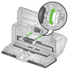
4. Reinstall the feed roller cover by positioning it around the paper present sensor, aligning the bottom edge of the cover with the scanner, and pushing it back into position until it snaps into place.
