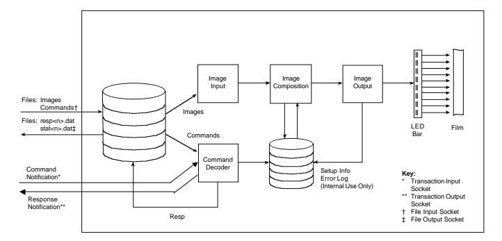
This diagram illustrates the internal flow of information and images through the Writer.
